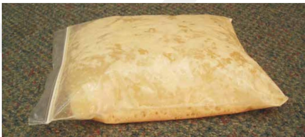
Photograph showing the inflated bag of Sample C after 20 minutes
